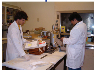
RSO technical assistants Jamie Dismukes (left) and Bobby Zhang carry out a routine radiation laboratory contamination survey using smears and a pancake Geiger-Mueller probe survey meter.
