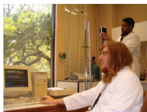
RSO technical assistant Nicholas Kubiak (left) and research specialist Nicholas Desselles perform leak test analysis of sealed radioactive sources using an alpha-beta proportional counting system.
